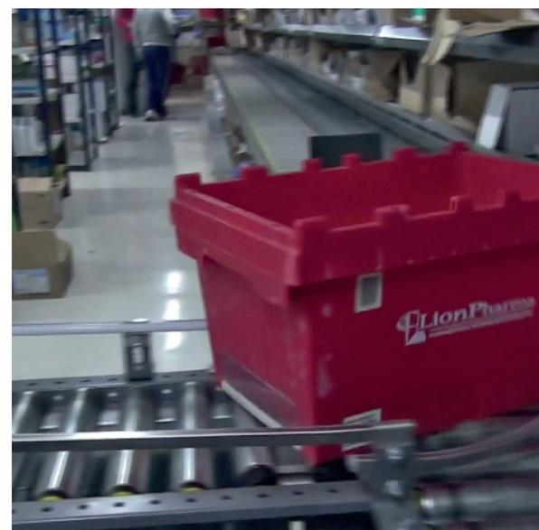
At the picking zones, operators collect the items of each order and place them in the respective crate. During this process, operators use wireless ZEBRA terminals to scan both crates and products thus ensuring correct collection of order items and at the same time send picking confirmation to the ERP.
