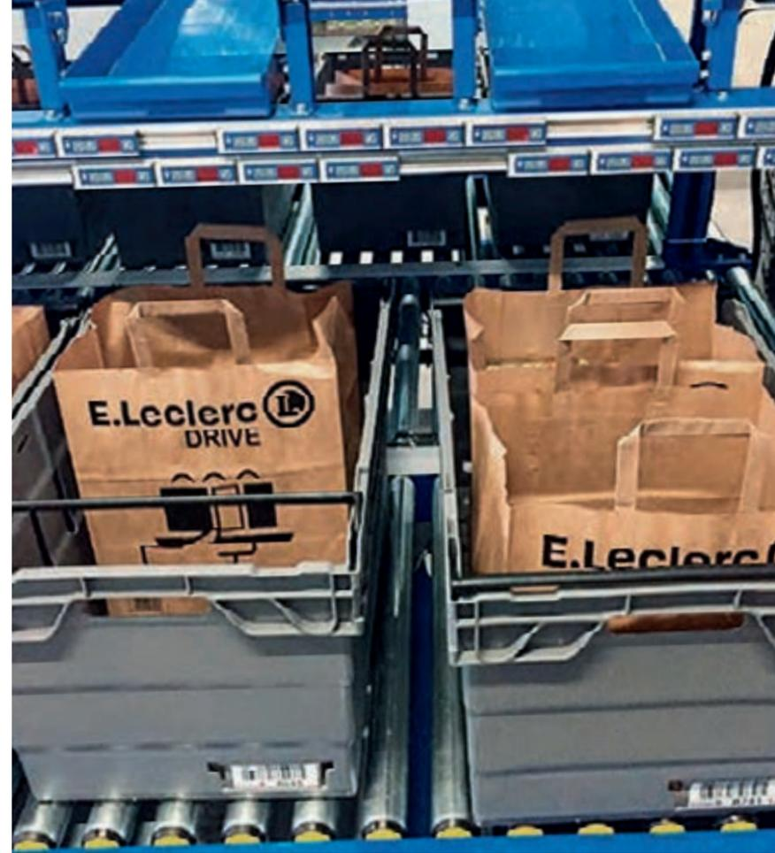
This saves a lot of energy and also reduces the noise level as well as the wear and tear on conveyor components. SegmentControl controls up to two zones of a conveyor. Each zone consists of a RollerDrive EC310,
